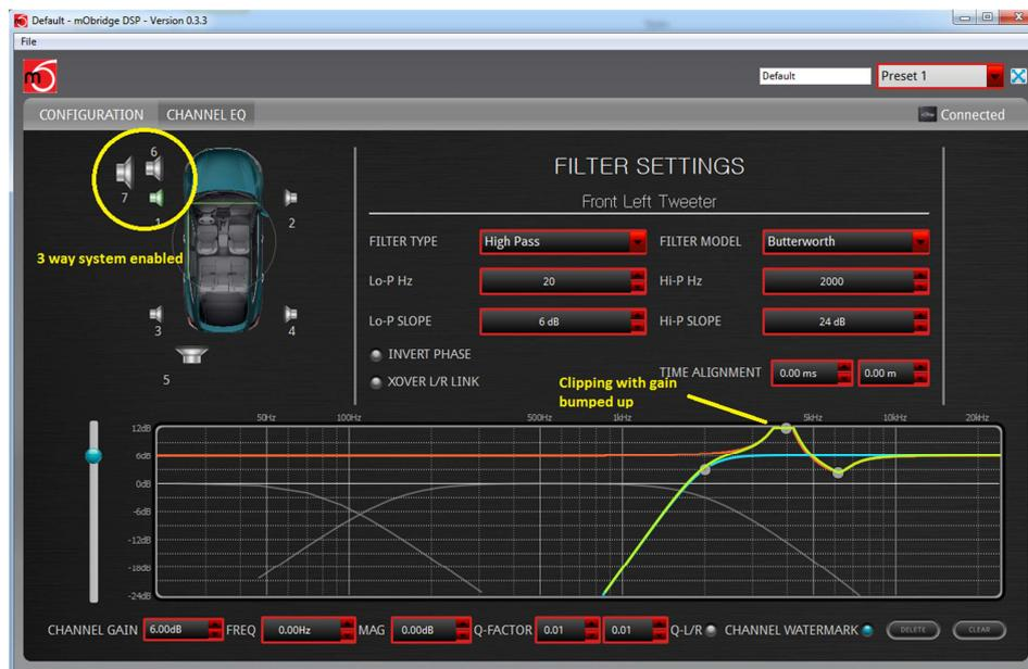
Figure 10 Channel Equalizer with mater mark
