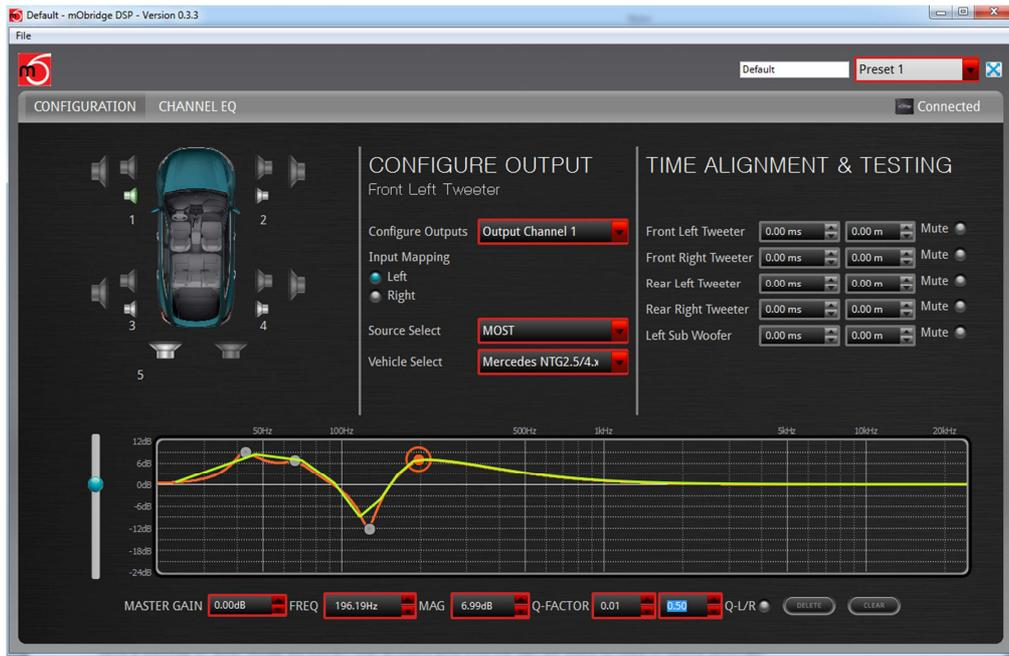
**Figure 12 Master Equalization**
