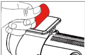
2. Remove the protective tape from the bracket.
